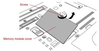
Figure 3-15 Removing the memory module cover
